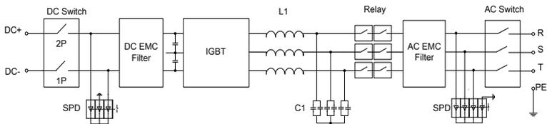
**Fig. 2-5** Circuit diagram of SG125HV
