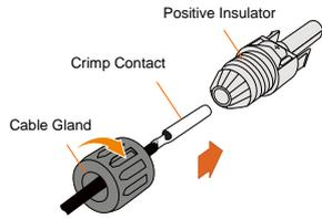
**Step 5** Screw the cable gland to front insulator with tightening torque 2.5...3 N·m.
