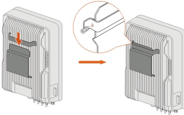
**Step 6 (Optional)** If you purchased a GPRS data acquisition module, install it to the communication interface of the inverter.
