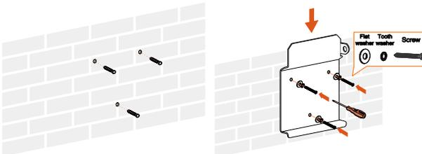
**Step 5** Lift the inverter above the backplate and then slide down to make sure they match perfectly. You can use the fastener set to lock the device.
