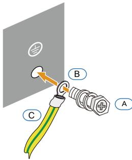
**Fig. 3-3** Second PE connection
