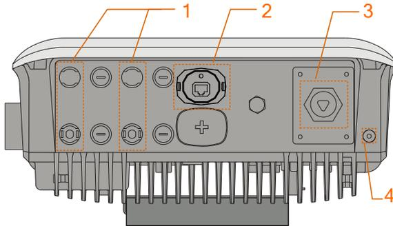
**Fig. 3-1** Cable connection area
