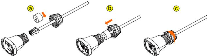
**Step 2** Insert connector of one cable end into COM terminal on the bottom of the inverter. Make connector and COM terminal engage and rotate clockwise.
