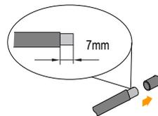
**Step 2** Assemble cable ends with crimp contacts by crimping pliers.
