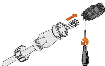
**Step 5** Pull cables outward to check whether they are firmly installed.
