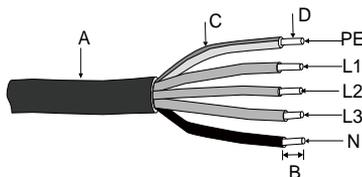
**Step 4** Fix all cables to the corresponding terminals by torque of 2.0-2.5N·m, according to markings on the connector with a screwdriver, especially the "PE" cable.
